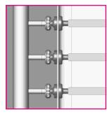
Vacuum tight feedthroughs for the connection nozzle of the heated inserts in the backwall of the vacuum chamber. The inserts and the distributor tube for the heating media are removable. For many years now VT vacuum drying ovens have proven themselves. The shelves/heated inserts of these standard vacuum drying ovens are removable.
