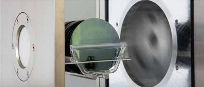
The system V10-G is designed for resist stripping of small batches.
