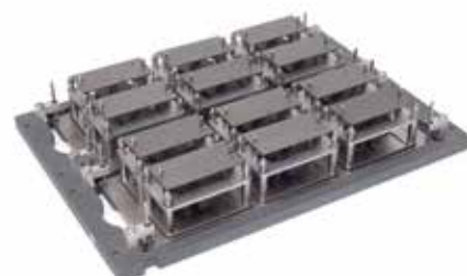
Carrier with fixtures for soldering of connecting contacts.
