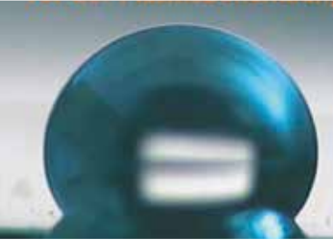
A hydrophobic polymer surface prior a treatment with low-pressure plasma.
