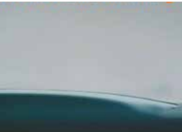
The same surface has hydrophilic properties after plasma treatment.
