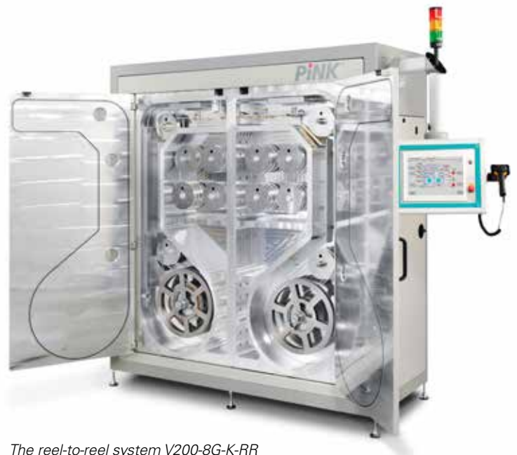
The reel-to-reel system V200-8G-K-RR cleans the surface of leadframes.
