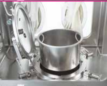
A mobile pressure nutsch with removable filter insert is integrated in the isolator.
