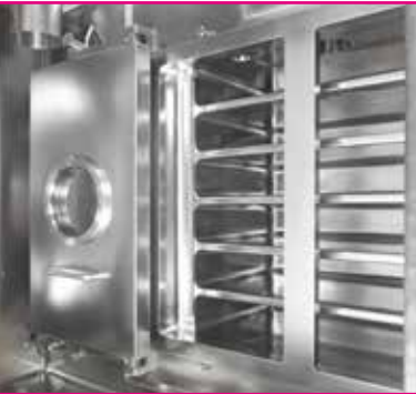
Integrated vacuum drying oven VSD with double-walled, jointless interior.
