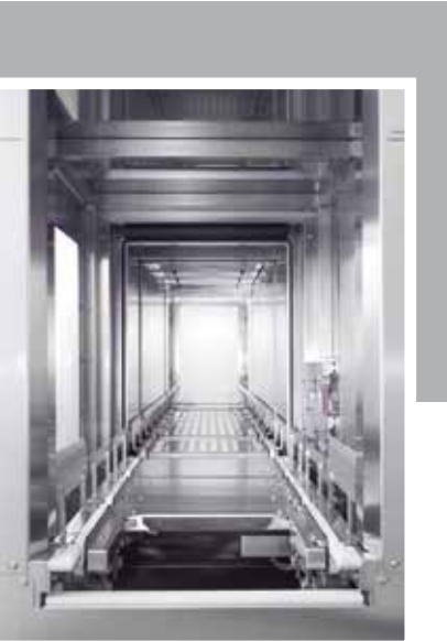
Inline system with circulating air heating zones and a vacuum drying zone.
