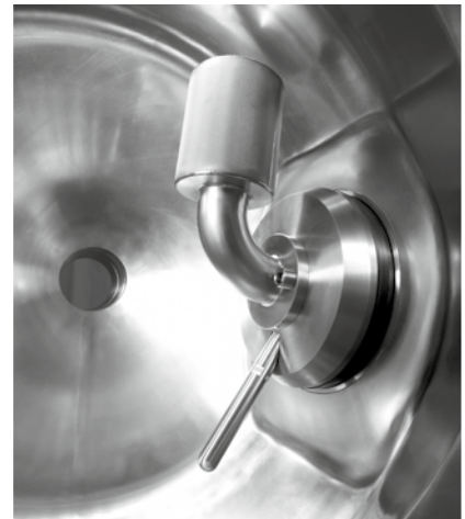
GMP-compliant drum interior with filter and product temperature sensor.
