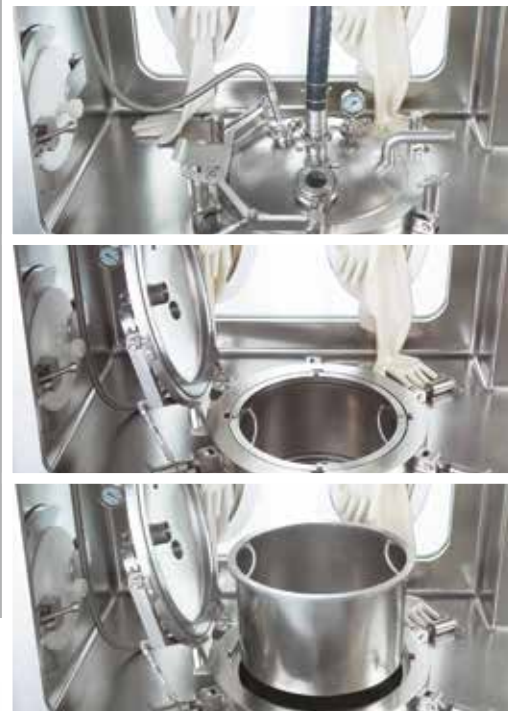
A pressure nutsch with removable filter insert is integrated in the isolator.
