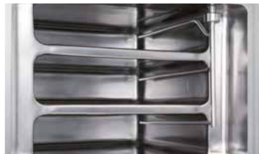
N 2 distribution manifold: Vertical distribution tube with gas guide lances in each charging chamber – for the controlled introduction of gases and for chamber ventilation.
