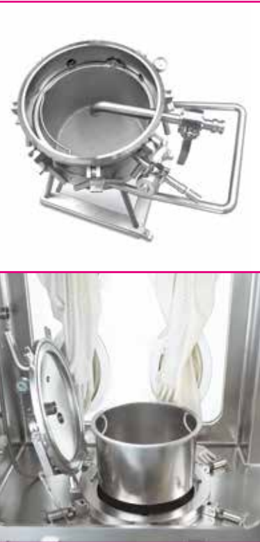
A mobile pressure nutsch with removable filter insert is integrated in the isolator.
