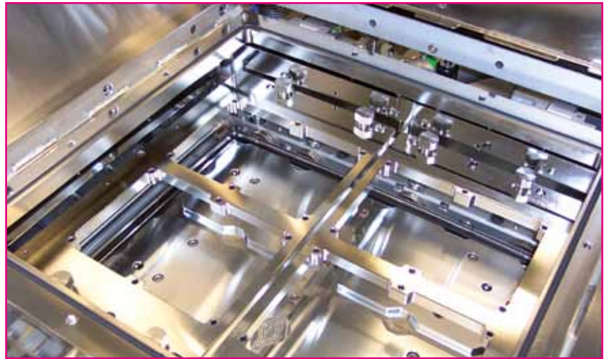
Carrier with integrated low-clamp frame for automatic fixture in the process chamber.
