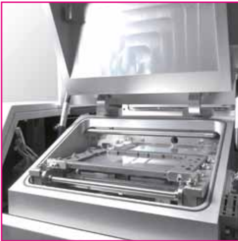
The VADU 100 system is provided with separate process zones for soldering and cooling.
