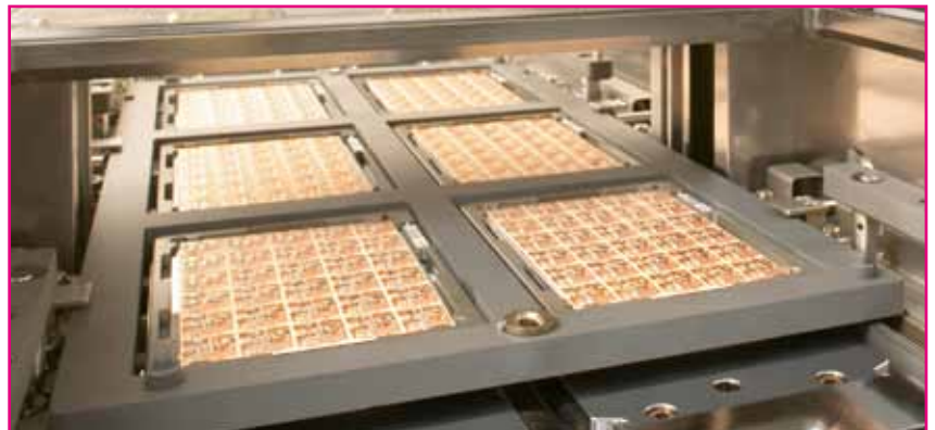
Carrier with base plates and 5 x 7" master cards.
