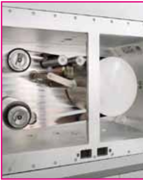
The process chamber with plasma source and winding mechanism.
