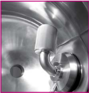
GMP compliant drum interior with filter and product temperature sensor.
